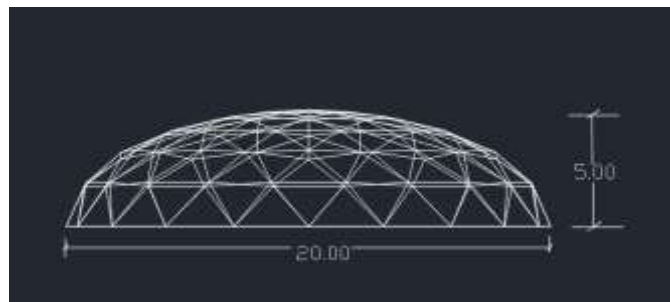
Fig.2.3: 4V,1/4 H to S Geodesic dome Model-4: 6V,1/2 H to S Geodesic dome
