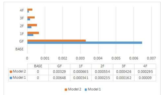
Fig. 6: Storey Drift in Y-direction
