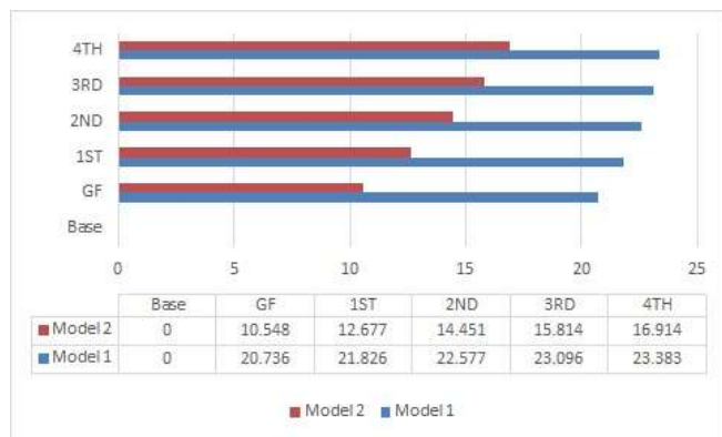
Fig. 4: Storey Displacement in Y-direction
