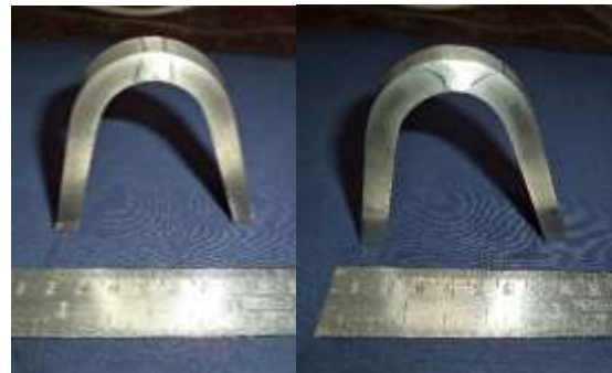
Fig. 3. Bend test specimen
