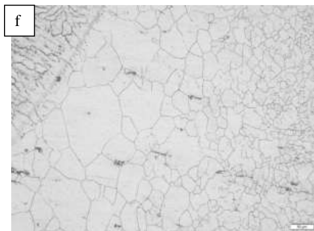
Fig. 12. Microstructure of HAZ of SS304H
