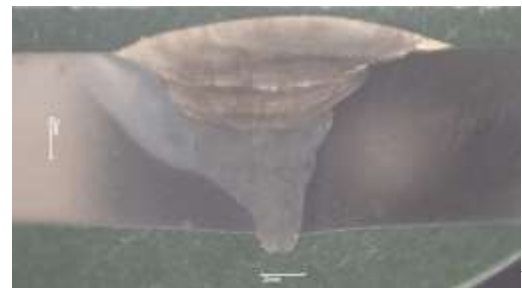
Fig. 6. Macro-etched weld joint
