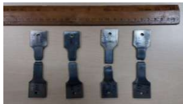
Fig. 4. Hot-Tensile test specimens
