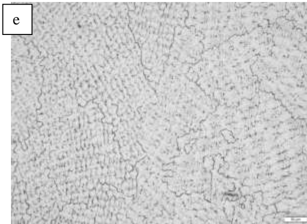
Fig. 11. Microstructure of weld metal
