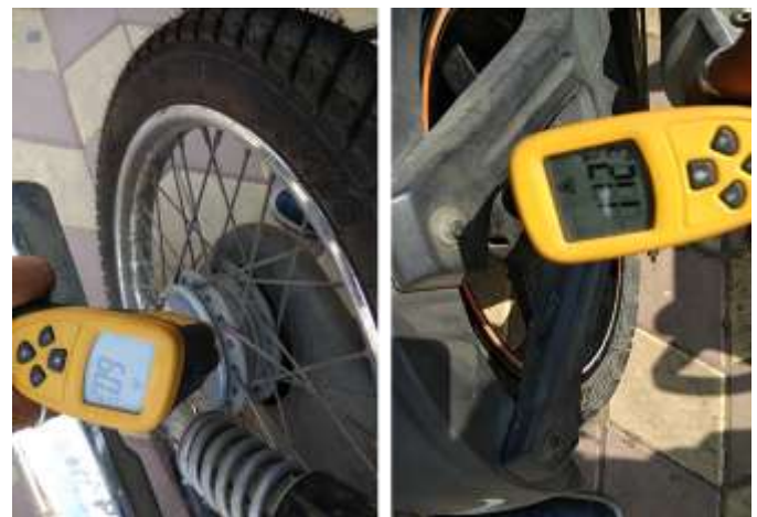
Fig -3.1: temperature rise in drum
