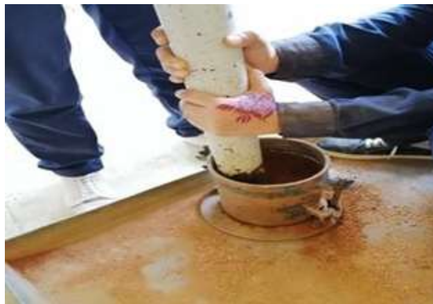
Fig.3: CBR mould 3.Unconfined Compressive Test
