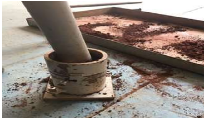
Fig. 2: Preparation of mould for proctor 2.California Bearing Ratio Test(CBR)
