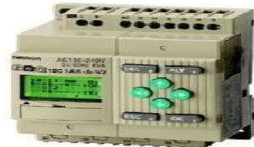
Fig- 5.1: PLC modules
