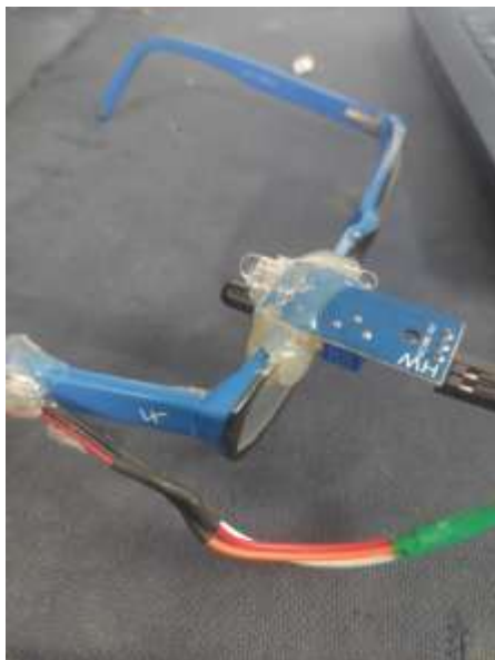
Fig -8: IR Sensor module mounted on spectacles
