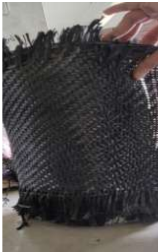
Fig.4.2: CFRP Wrapped specimen
