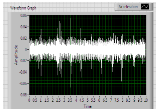
Fig -4: Vibration signatures in LabVIEW software for 900 RPM and 0mm eccentricity
