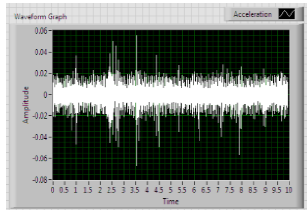
Fig -3: Vibration signatures in LabVIEW software for 700 RPM and 0mm eccentricity
