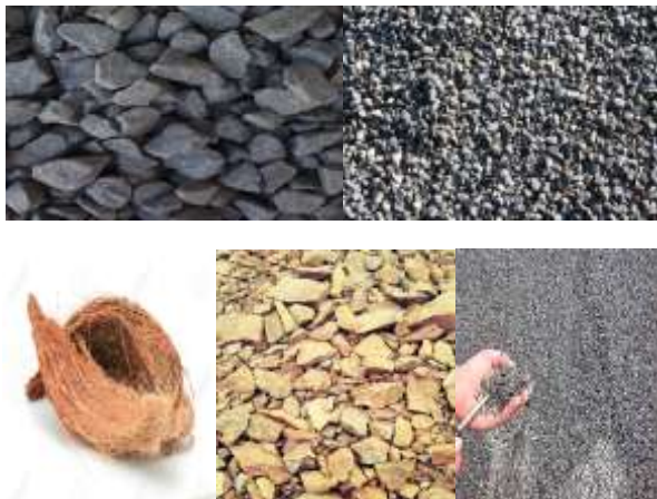
Fig.1: Material used as filter media (Gravel, sand, coconut shell and Coconut husk, basalt rock, rock dust)
