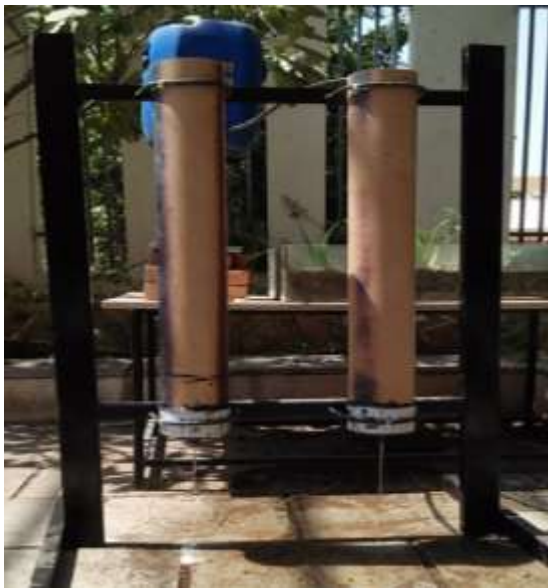
Fig 5: Working model of Soil Bio-Filter
