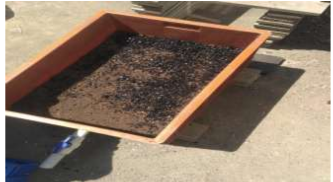
Fig 11 Shows Layer of GAC above river sand
