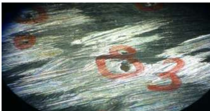
Figure 5. Pitting observed under the microscope
