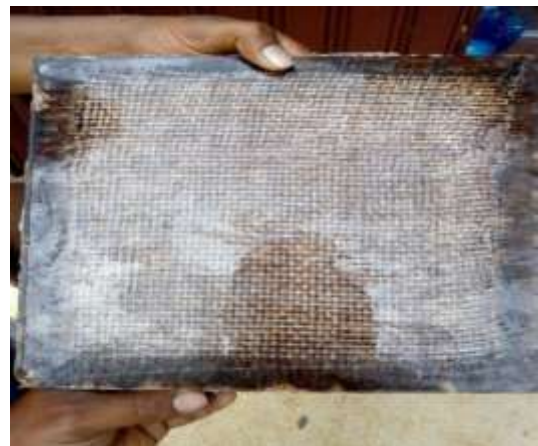
Fig -2: Prepared composite material with 5% of coconut shell powder
