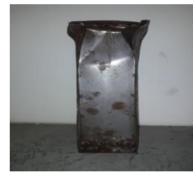
Fig 12: Failure of welded column
