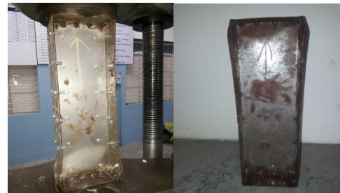
Fig 11: Failure mode of Bolted column and Welded column
