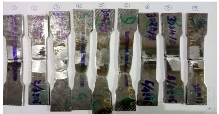
Fig-1:- Specimens after Tensile Test.
