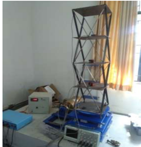
Fig -3: Diagrid model set on horizontal shake table
