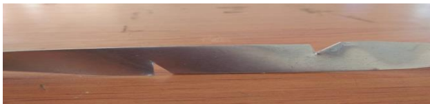
Fig.2. Right angle triangle twisted tap arrangements in the twisted tap with twisting ratio of 1:2
