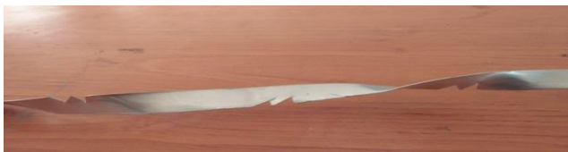
Figure.3. W-Cut Twisted Tape arrangements in the twisted tap with twisting ratio of 1:2
