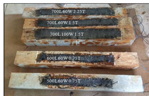
Fig-8: Strengthened beams
