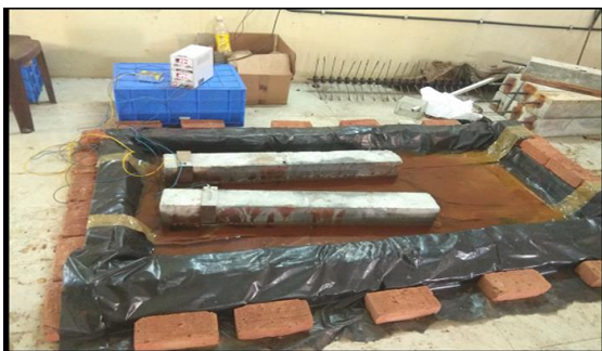
Fig -5: Corroded beams in the test set up
