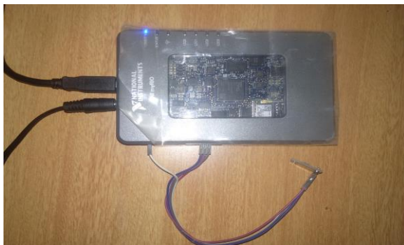
Fig -2.2: Circuit setup of MyRio-1900 & ADXL 335
