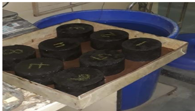
Figure 1: Marshall specimens for different bitumen percentage
