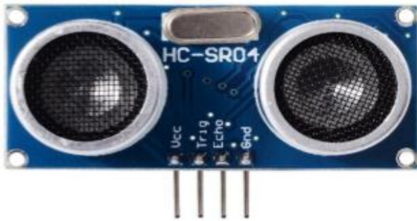
Fig 2: HC-SR04 Ultrasonic Sensor
