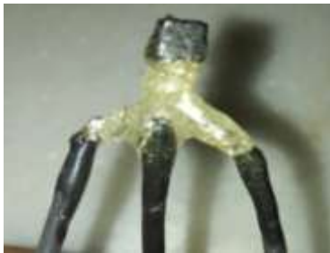
Fig -1: Sensing module after preventive coating
