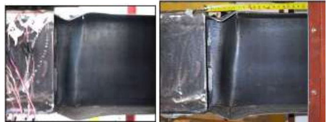
Fig -6: Starting and Fully Developed Crack
