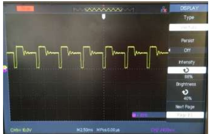
Fig. 4.6 Output voltage waveform of proposed bridgeless boost PFC rectifier
