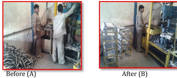
Before (A) After (B) Figure 8: Bush Inserting and Drilling Workstation
