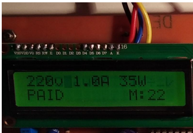
Chart -2: Volt, Ampere, Watt show in Lcd Display
