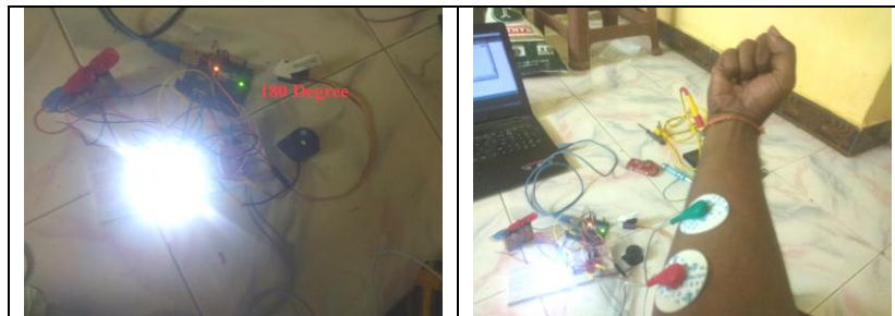
Fig -8: Servo Motor "180 Degree position" at forearm flex condition
