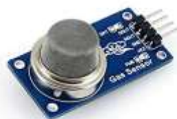
Fig -4: Gas Sensor
