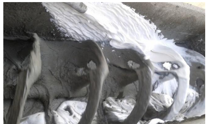
Fig.5 Mixing of CLC with foam
