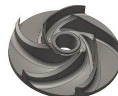
Figure 3: Existing impeller - 3D model using CATIA software
