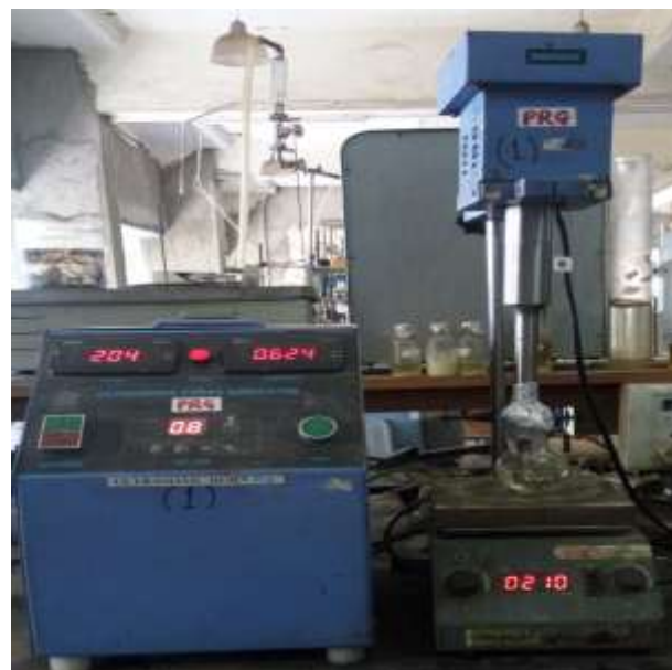
Fig 1: Pictorial representation of the experimental set up for the Ultrasound assisted synthesis of biodiesel.
