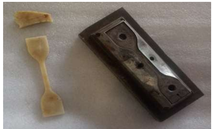
Fig.3 Specimen for testing
