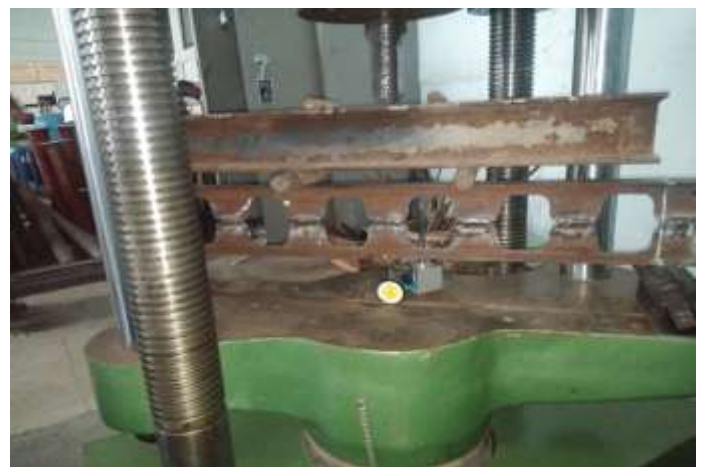
Fig- 8: Test setup for castellated beam with sinusoidal opening.
