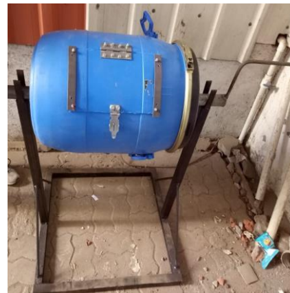
Fig 1 Rotary Drum Composter
