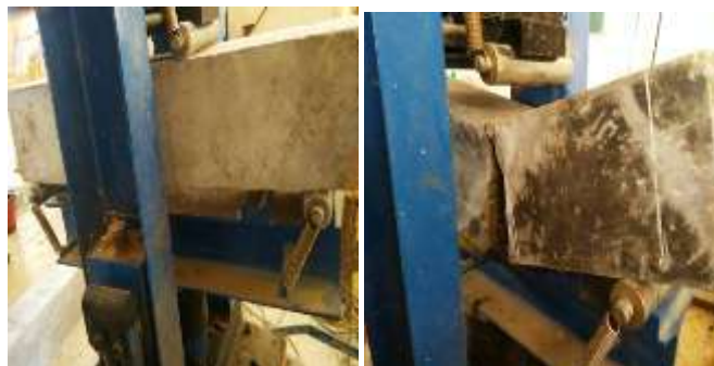
Fig 3: Flexural testing on beam
