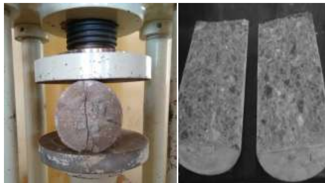
Fig 4: Split tensile strength testing on cylinder
