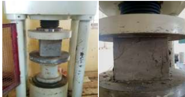
Fig 2: Compression testing on cubes
