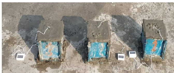
Fig -2: An Image showing Casted cubes including sensors
