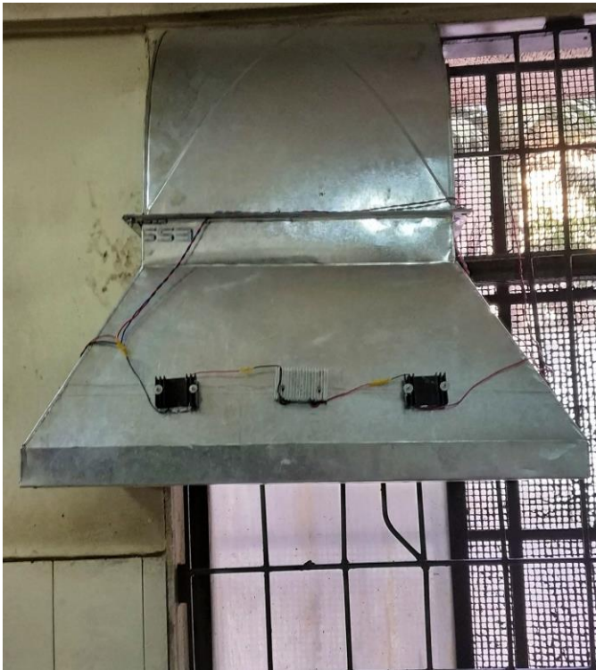
Fig - 3: Position of Peltier module sandwich
