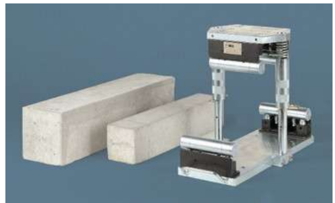
Figure 2: Test for Flexural Strength of Concrete
