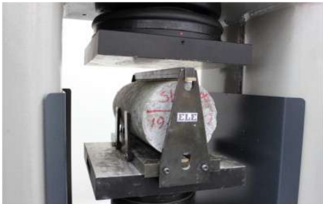
Figure 3: Test for Splitting Tensile Strength
