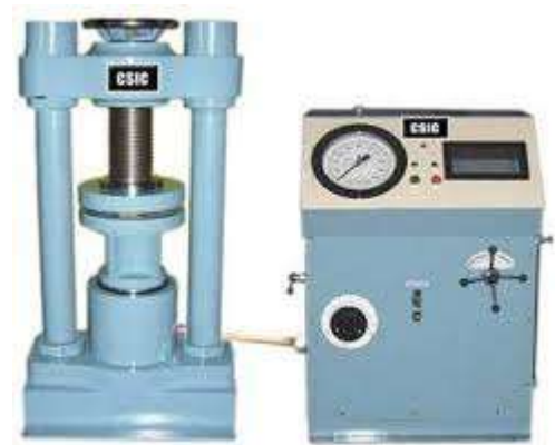
Figure 1: Test for Compressive Strength
