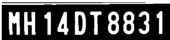
Fig -6: Segmented & Extracted Number Plate
