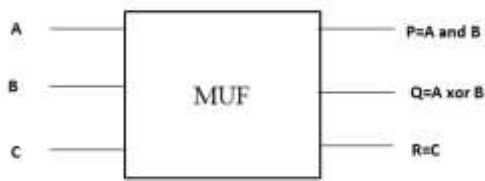
Fig -1: Reversible MUF Gate
