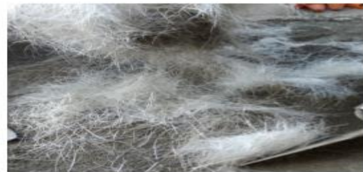
FIG: 1.1 MIXING OF PVA FIBER IN CONCRETE
