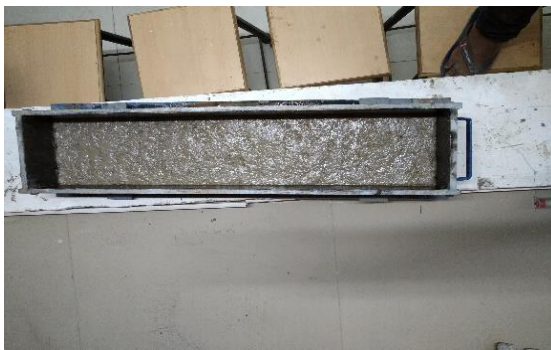
FIG: 2 CASTING OF ECC CONCRETE IN SLAB
