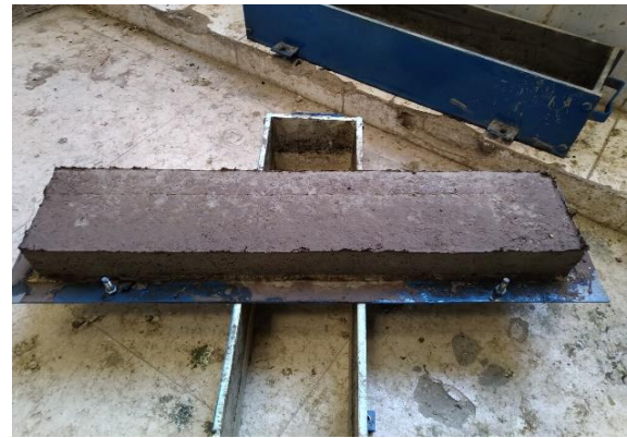
FIG: 3 ECC CONCRETE IN SLAB WITH 60mm THICKNESS AFTER DEMOULDING
