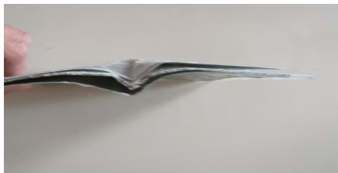
Fig-5 Delamination of metal faced specimen
