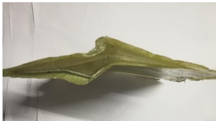
Fig-4 Delamination of fiber faced specimens
