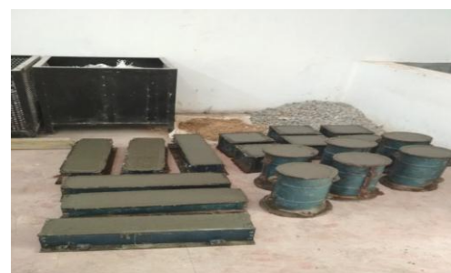
Fig 3: Casting of Specimen
