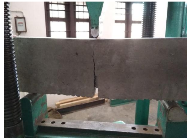
Fig -4: Typical Photograph of Failure of Notched Beam Specimens under Three- Point Loading
