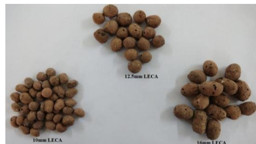
Fig -1: Typical Photograph of Light Weight Expanded Clay Aggregate
