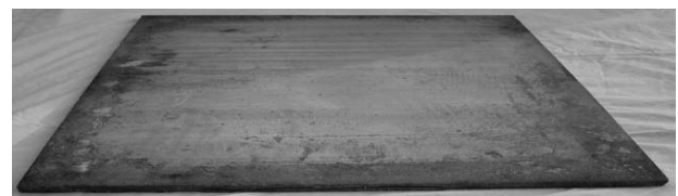
Fig 2 A specimen for sample making was a panel with the dimensions of 680 mm × 580 mm × 13 mm
