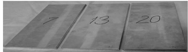
Fig 1 Thermally processed and machine for FSW 180 mm x65mmx5mm
