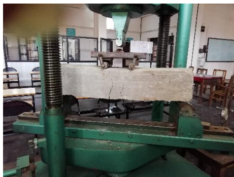
Fig-1: Testing of control specimen : Two point loading
