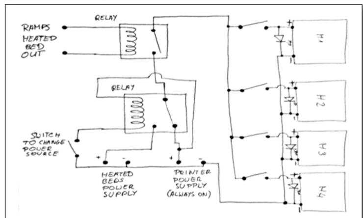
Figure 6: Heat Bed Circuit[11]
