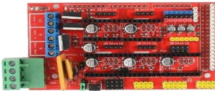
Figure 3: RAMPS 1.4 Control Board
