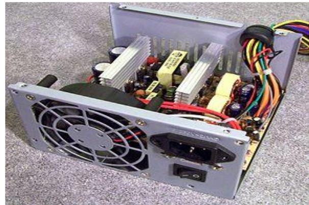
Figure 2: power supply unit
