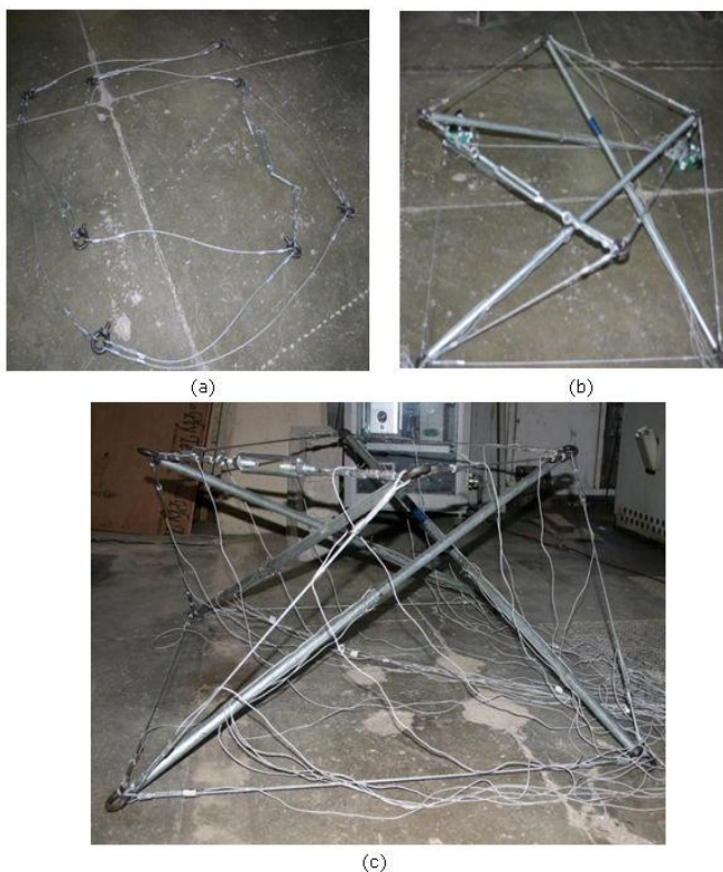
Figure 5: Different Stages of Deployment of Tensegrity Structure in Cable Mode, (a) Stage 1, (b) Stage 2, (c) Stage 3
