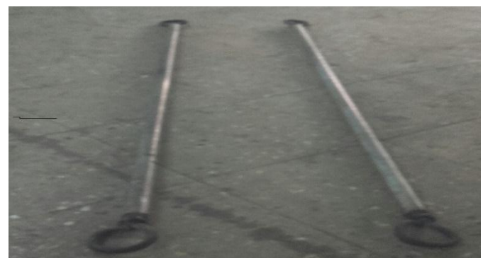
Figure3: Eye bolt joint with GI pipe
