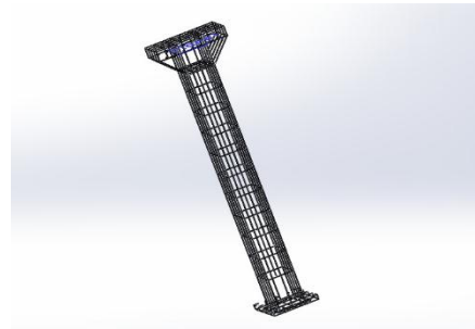
Figure 4: Reinforcement details of square column
