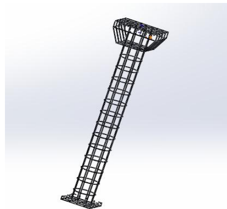
Figure 5: Reinforcement details of circular column
