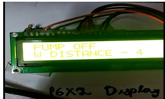
Fig. 5.3 Output: Pump Off
